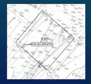
Located near the western corner of A-470, the C.G. Allen #14 well mud log shows oil shows at approximated 4,277' - 4,293'.
